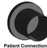
The main breathing hose (22mm) is connected to the large connection port.
